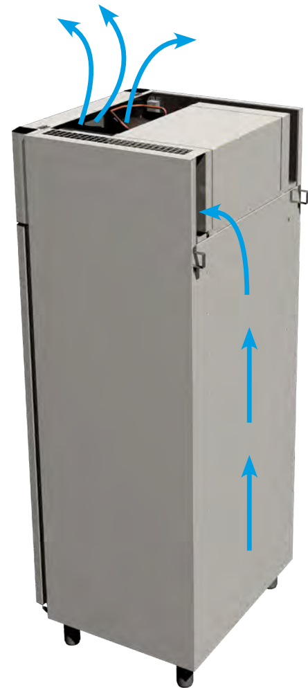
DC and DF condenser air circulation
